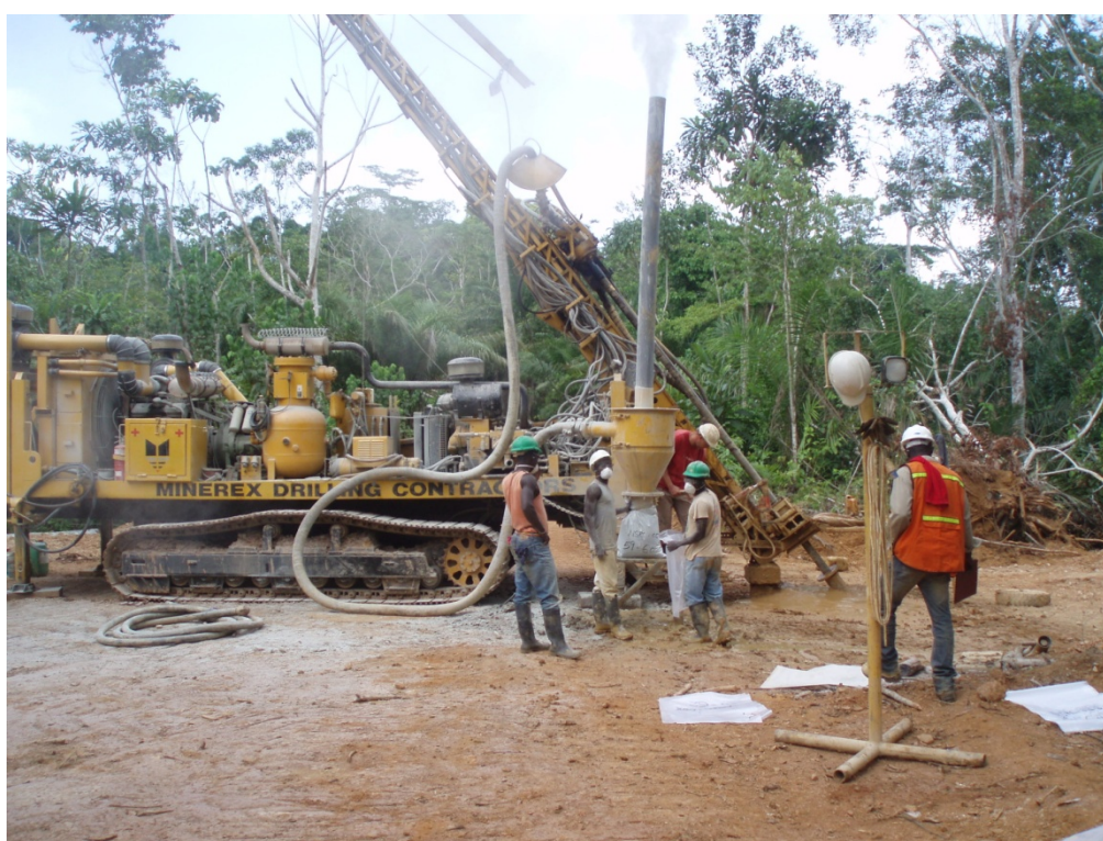
RC Drilling at CTP Project June 2009
